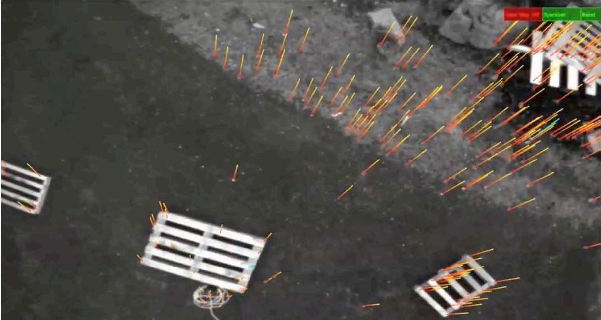
What the camera on board the helicopters sees: corner features extracted and matched between two frames.
